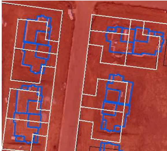
Figure 16: Foundations Do Not Match Parcels
