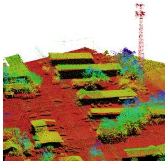
*Figure 1: Dense LiDAR – Note the Power Lines*
