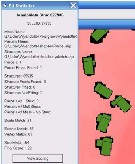
Figure 19: Sketch Scoring Against LiDAR Mask
